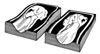
**Demold--** After the rubber has fully cured, remove the model from both halves. Assemble the mold by aligning the positive and negative keys. Use heavy rubber bands or mold straps to hold both halves together when casting into the mold.
