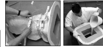
The pieces of the support shell are then assembled. They should align and fit together easily. Elastic bands or "mold straps" are then used to secure the pieces, and will hold everything together during casting. Matrix<sup>TM</sup> NEO<sup>TM</sup> is then mixed (as directed) and poured into the mold cavity.
