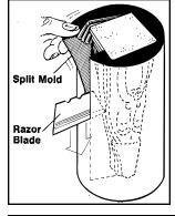
After the rubber has completely cured and the containment field has been removed, use a razor knife to carefully cut the mold down one side and half way across the bottom, on a line that will facilitate ease of removal.
