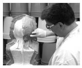
The mixed Plasti-Paste is then brushed or trowelled onto a section of the model and up against the installed clay shims. Care should be taken to avoid having "thin" areas of the shell. Edges of the shell should also be thickened to secure maximum strength
