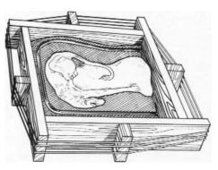
Apply a sealing agent and release agent as directed (depending on the mold rubber you are using) over the model, clay and sidewalls
