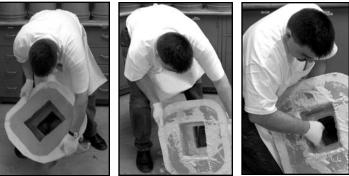
The mold is rotated by hand to build a uniform coating on the mold surface. The working time of this material is about 10 minutes, and the mold is rotated until the material no longer flows. A second batch of Matrix<sup>TM</sup> NEO<sup>TM</sup> is mixed and poured into the mold cavity, and the mold is again rotated for about 10 minutes. This layer of plaster bonds to the first. This process is repeated twice more, and an ultimate thickness of about 3/8" (1 cm) is attained.
