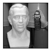
• Apply a light mist coating to the model surface and surrounding forms including mounting platform.
