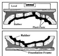
When the rubber has cured, build a level foundation frame on the shell. Mix *Plasti-Paste<sup>m</sup>* and build a suitable support for the foundation frame. Using a carpenter's level, build the framework so that the mold will be perfectly level when casting into it.
