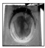
After thorough mixing, pour resin into the mold at the lowest point. Letting the mixture rise from the lowest point in the mold will displace air and help minimize bubbles in the cured casting.
