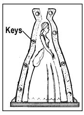
When the plaster has set, remove the cardboard templates. What remains is the first half of the support shell. Using a knife or screwdriver, carve out circular notches-or registration keys--at regular intervals around the inside perimeter of the shell. As we will see later, these "keys" provide a locking mechanism when both halves of the shell are complete and everything is assembled for casting.
