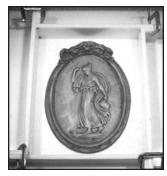
Note that there is ample room surrounding the model (at least 1/2" or 1 cm in all directions, including up and over the highest point of the model). These spaces between themodel and the walls of the mold box define the wall thickness of the finished mold. The space above the model defines the foundation thickness of the finished mold.
