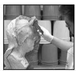
the mold rubber and shim, Plasti-Paste is measured, mixed and applied to form the second segment of the support shell. Allow the second segment of the support shell to set up and harden.
