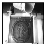
You will notice tiny air bubbles rising and dissipating on the surface. You can further dissipate these bubbles by lightly passing a heat source (hair dryer or heat gun) over the surface.
