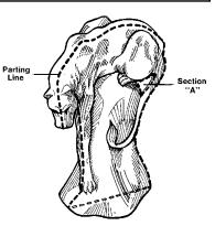
The parting line is inscribed (as illustrated) and the model is laid horizontally into a moldbox. Modeling clay is then built up from the platform to the parting line. The model should be as level as possible and parallel to the base.
