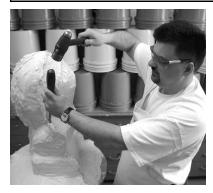
Using a hammer and screwdriver, lightly tap and create perforations along each parting seam. The screwdriver is then inserted into the perforations and the shell segments are gently pried away from the model and each other.
