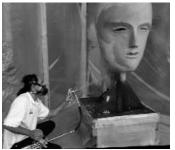
Mold Rubber can be applied by pouring, brushing or spraying onto a model.
