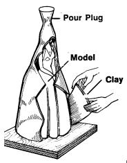
The next step is to identify or "map out" where the segments of the support shell will be applied. The number of shell segments depends on the complexity of the model (angles and undercuts). This model is relatively simple and therefore requires a two-piece support shell.
