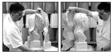
The visual mapping process (plan of attack) done prior to applying the mother mold has paid off, as the three shell segments are easily removed. Carefully place each segment aside until all three portions of the support shell have been removed from the model.
