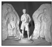
**MOLDMAKERS TODAY** still use a variety of materials, but a majority uses one of four different flexible rubber products for the following reasons: 1) these rubbers **reproduce exact detail**, 2) flexibility allows for **easy removal (demold)** from the original model and the cast piece, 3)
