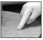
room temperature) until *"tacky."* Tacky means that the rubber has started to cure and is no longer "wet." It is sticky to the touch, but will not come off on your finger (use only a gloved hand or a spatula to touch the rubber). **Note:** *Colder temperatures will prolong the cure time, while warmer temperatures will accelerate it.*
